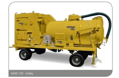
Big size trolley-mounted unit. Standard version driven by a 6-cylinder Turbo-charged Diesel engine, water cooled and 120 L fuel tank. Large filter mounted in the vacuum unit automatic mechanical shaker. 400 L fine dust compartment. Hydraulic system for discharging container. Container fitted with highly efficient cyclone head. D100mm or D120mm suction inlet.
