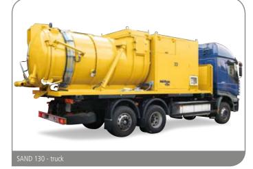
Big size truck-mounted unit. Standard version driven by a 6-cylinder Turbo-charged Diesel engine, water cooled and 82 L fuel tank. Large filter mounted in the container with automatic mechanical shaker. Hydraulic system for discharging container. Container fitted with level sensor. Double suctions inlets D100mm or D120mm. Side room for placing accessories.
