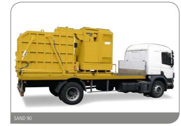
Medium size truck-mounted unit. Standard version driven by a 4-cylinder Turbo-charged Diesel engine, water cooled and 85 L fuel tank. Available also with electrical motor. Large filter mounted in the container automatic mechanical shaker. Hydraulic system for discharging container. Container fitted with level sensor. Double suctions inlets D100mm.
