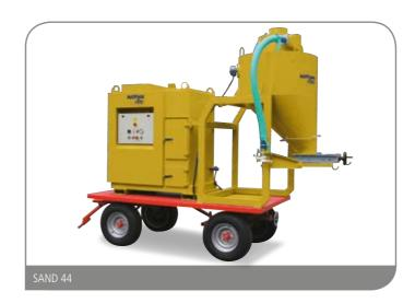
Small unit trolley-mounted and very mobile. Standard version driven by a 3-cylinder Diesel engine, water cooled and 54 L fuel tank. Available also with electrical motor. Large filter mounted in the vacuum unit with automatic mechanical shaker. 150 L Fine dust compartment. Many inspection doors. 1 m3 hopper with level sensor, cyclone head and D250mm discharge valve. D80mm sucking inlet.
